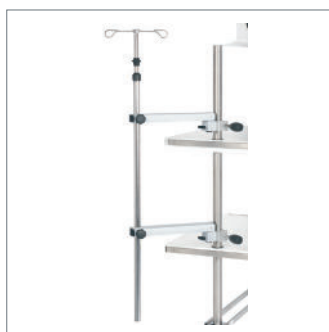
Telescopic IV pole, 4 hooks on arm with 300 mm horizontal extension Load max : all 32 kg and 2 kg / hook
