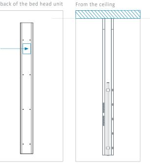
The SIMPLE CARE is quick and easy to install thanks to its screw-mounting system via the back of the strip.
