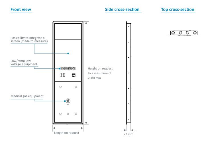
The MULTIDYS panel is made-to-measure. Manufactured in stainless steel or powder coated steel RAL 9016, it enables the distribution of low, extra low voltage and medical gases.
